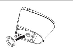
2. Align the ceramic drain with the drain hole on the ground, and press down to make the wax ring fully contact with the ground.
