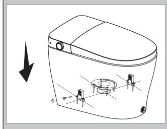
3. Fix the two sides of the ceramic with two bolts, and finally install the cap.
