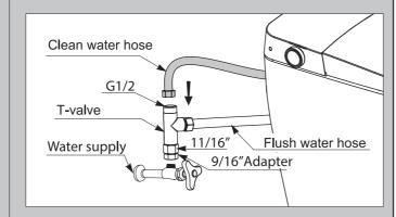
6. Connect the T-valve to the water supply and tighten.
