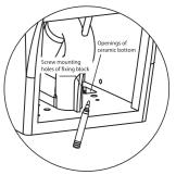
1.Put the flange on the drain hole, and fix it on the ground with four bolts. Then Seal the flange with glass glue.
