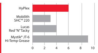
Elongation is a measure of the adhesive-cohesive "stringiness" of a grease and indicates its ability to effectively travel through moving systems and create a protective coating.
