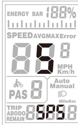
SPS indicates the speed sensor setting. It can be set according to the number of magnet heads mounted on the wheel of the e-bike, and the setting range is 1-9. Modify it by pressing UP/DOWN. Hold MODE to confirm and return to the personalized parameter setting interface. The factory default value is 1.
