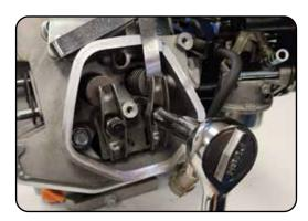
The engine intake and exhaust valve clearance should be checked and if necessary adjusted every 300 hours of use or 12 month period, whichever comes first.
