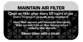
Routine maintenance of the air cleaner helps maintain proper airflow to the carburetor. Check that the air cleaner is free of excessive dirt after every use.
