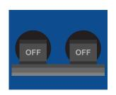
**Step 7:** Once the generator is running, turn the main breaker to ON and plug devices in.
