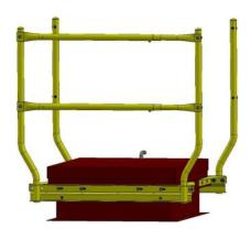
**STEP 6** — Slide rail extensions in to mid and top railing assembly and attach to upright using (A) 2-1/2" x 3/8"-16 Button-Head Cap Screws.
