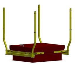
**STEP 5** — Attach front side mid and top rail assembly to upright using (A) 2-1/2" x 3/8"-16 Button-Head Cap Screws.
