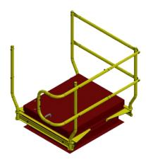
**STEP 8** — Slide rail extensions into mid and top railing assembly and attach to upright using (A) 2-1/2" x 3/8"-16 Button-Head Cap Screws.
