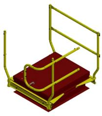
**STEP 7** — Attach opposite side mid and top rail assembly to upright using (A) 2-1/2" x 3/8"-16 Button-Head Cap Screws.
