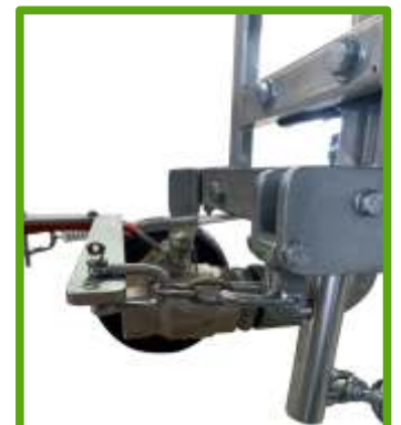
Pic 6. Handle locked into quick release mechanism
