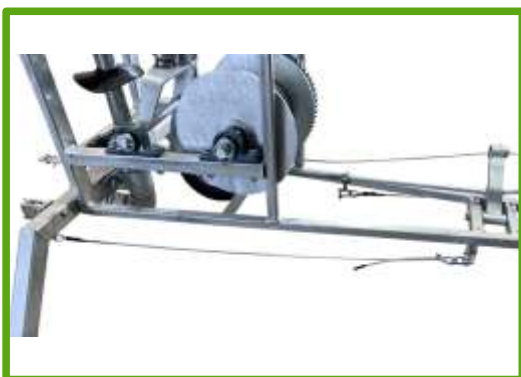
Pic 4. Connection between actuator and quick release mechanism
