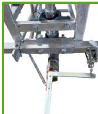
Pic 5. Shows mechanism 'loaded'. Valve is in the open position
