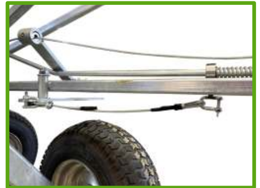
Pic 3. Connection between brake arm and actuator
