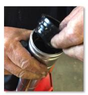
5) Drain the oil into a clean tub so it can be reused.
