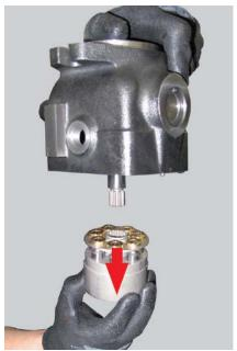
3. Remove the snap ring and remove the shaft, then replace shaft seal.
