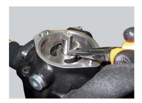
2. Remove the four screws to remove the housing (use a 6mm Allen key), then remove house, distributor, rotary kit, valve plate....
