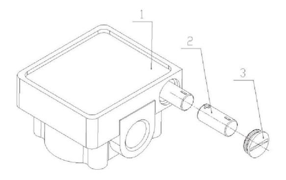
When the battery signal is flashing on the display, change the battery.
