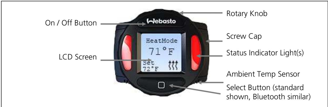
**Interface Description – SmarTemp Control 3.0 Panel (Coolant Heater)**
