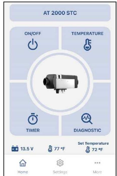
**Note:** Heater cannot be turned on with SmarTemp 3.0, if equipped, when attempting to connect with Webasto Thermo Test (WTT) via the diagnostic connector. When WTT is connected, the heater must be operated through the WTT interface.
