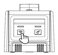
2.5 Press and hold **5 seconds** of WIFI button until the **indicator light blinks once per second.**
