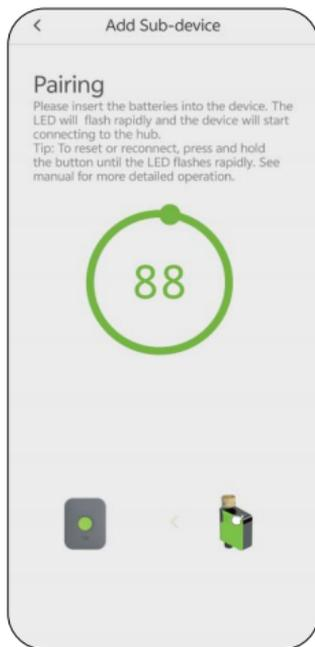
**NOTE:** The water timer can be paired with a smart hub or Bluetooth. Use a 2.4GHz WiFi to connect the hub and router, then pair the timer with the hub via Bluetooth. Please make sure your phone's Bluetooth function is on for better pairing.
