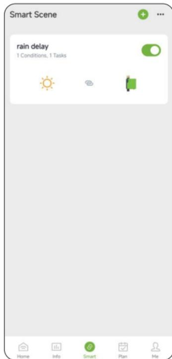
**For example:** The picture on the right shows that when the weather in New York is heavy rain, the valve of the HTV107B wireless irrigation timer will be automatically closed, and watering will be delayed for one day.
