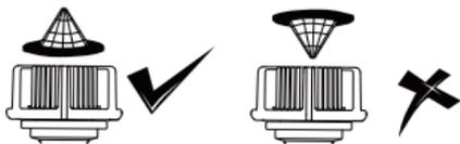
**Please install the filter correctly (as shown left) and keep it clean to achieve a better filtering effect.**
