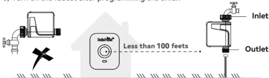
**Tips:** If the connection between the timer and the faucet or hose is not tight or is leaking, wrap more Teflon Tape (thread seal tape) around them to secure the connection.
