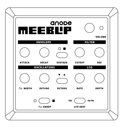
LFO RATE determines the speed of the Low Frequency Oscillator (LFO). Turned all the way down, the LFO is off.
