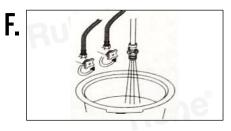
Turn on the hot and cold water source and let the water flow out for about a minute.
