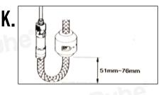
As shown in the picture, adjust the weight to the proper position and lock it.
