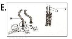
Link and lock the hose (6) to the water source. Connect the hose with the sticker (7) to the cold water
