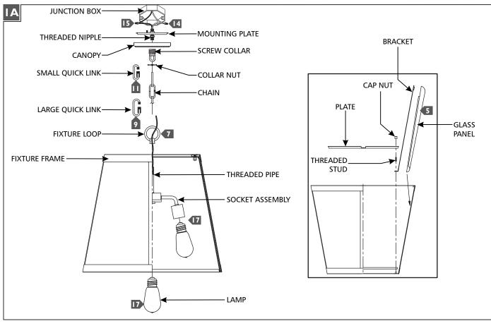
If necessary, screw the short end of the threaded nipple tightly onto the mounting plate and the screw collar onto the threaded nipple.
