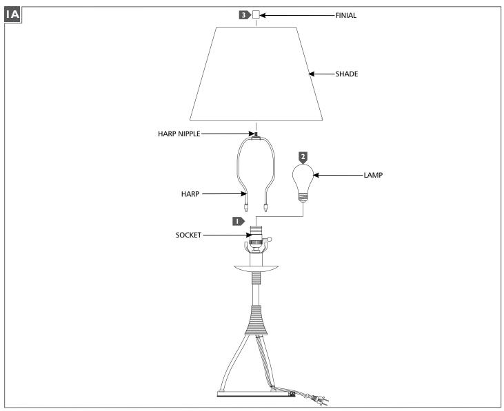
Install the harp by inserting it into the yoke.
