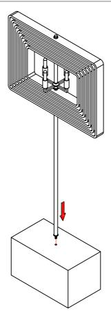
•Tilt the base and install the lower poles underneath by securing with hex nuts, plain washers and lock washers provided. please see sketch below.
