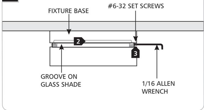
2 Place the glass shade into the fixture base until the grooved section of the glass shade is completely inside.
