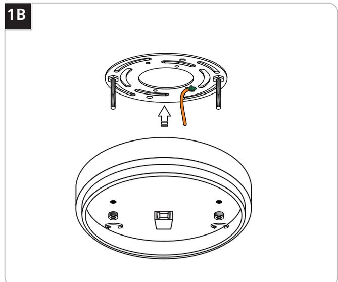
**3** Remove the mounting plate from the assembly by unscrewing the two knurled nuts.
