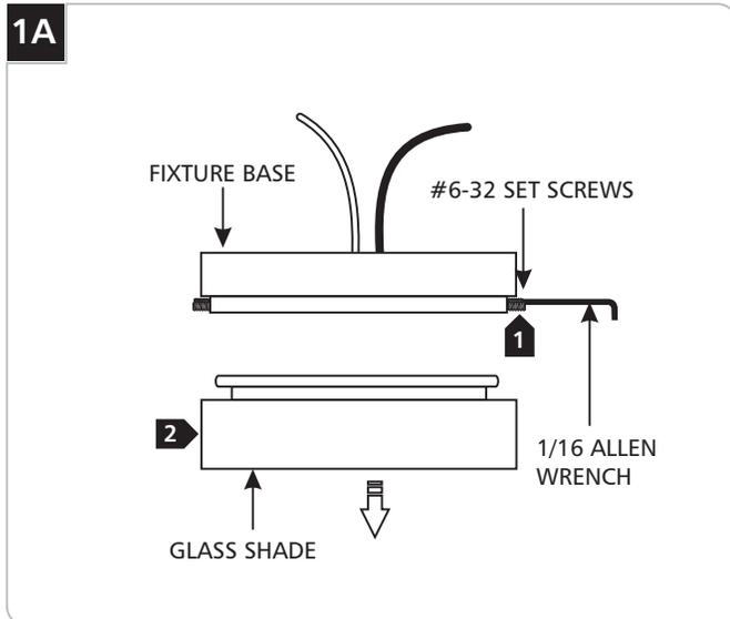
**1** While supporting the glass shade, loosen (**Do Not Remove**) all the #6-32 set screws on the fixture base with the 1/16 Allen wrench.
