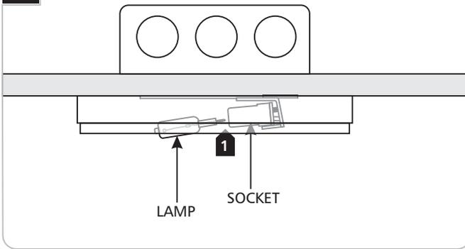
**CAUTION:** To reduce the risk of a burn or electric shock during relamping, disconnect the power to the fixture.
