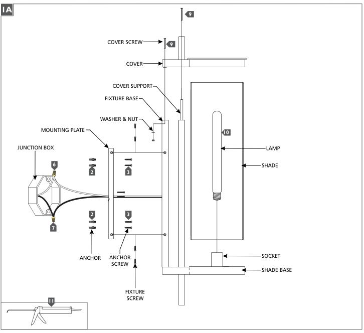
Temporarily install the mounting plate to the junction box
