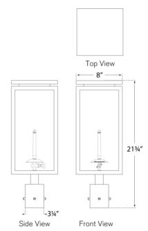
Gas light fixture supplied with  $_{3/16^{\circ}}$  copper gas line and  $_{3/16^{\circ}\times1/4^{\circ}}$  gas line adaptor
