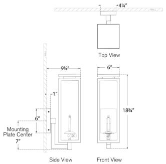
Gas light fixture supplied with  $_{3/16^{\circ}}$  copper gas line and  $_{3/16^{\circ}\times1/4^{\circ}}$  gas line adaptor
