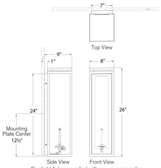
Gas light fixture supplied with  $_{3/16^{\circ}}copper$  gas line and  $_{3/16^{\circ}\times1/4^{\circ}}$  gas line adaptor
