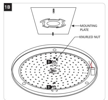
Remove the mounting plate from the fixture base by unscrewing the two knurled nuts.
