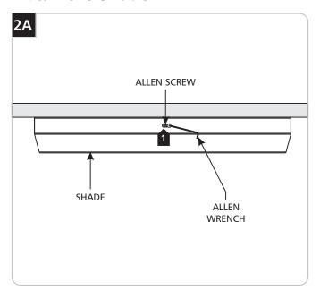
1 Align the holes on the shade with the holes on the fixture base and reinstall the two Allen screws using the Allen wrench.
