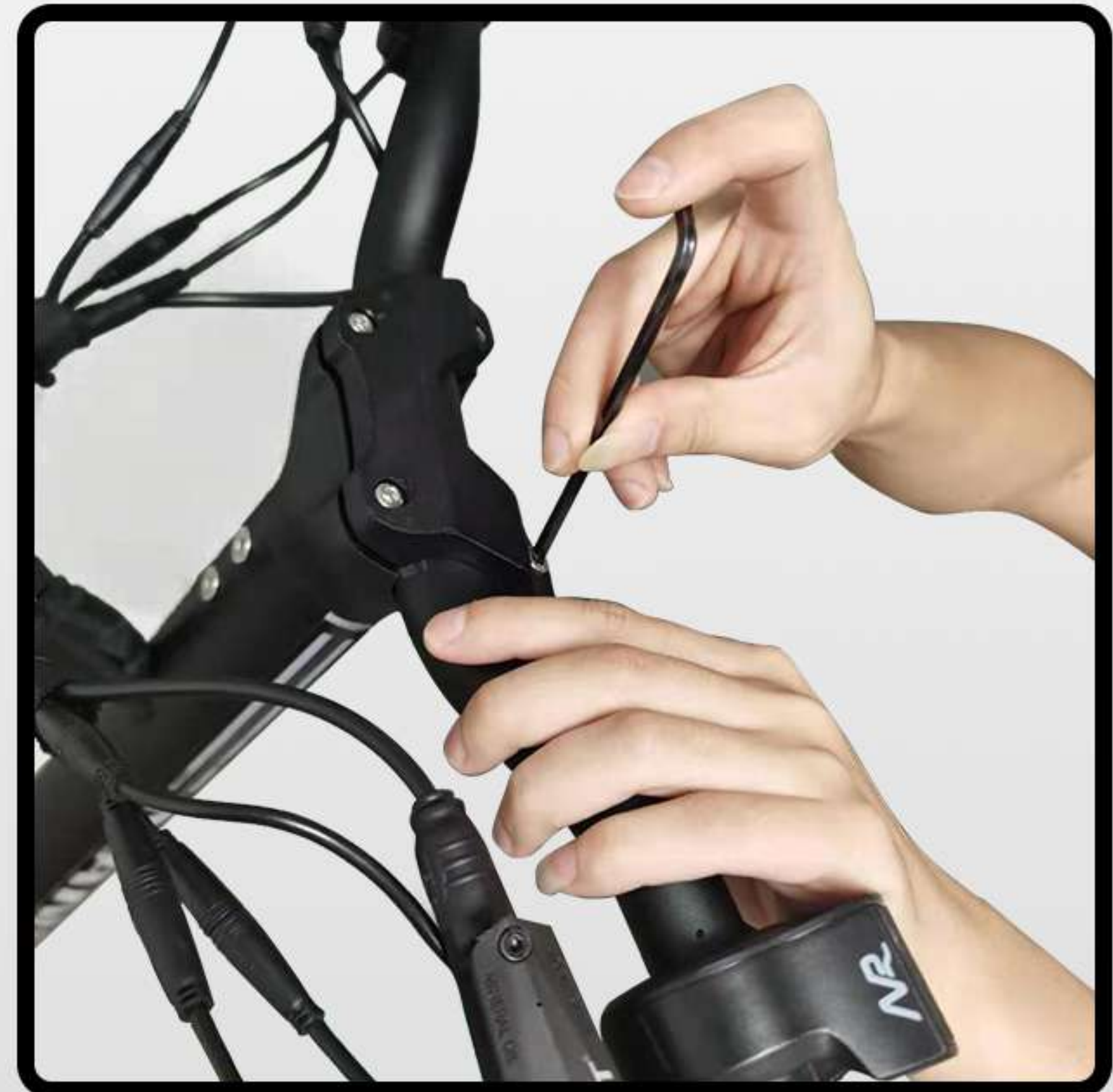
② After aligning the handlebar with the center mount, replace the cover mount, and tighten the fixing bolt.
