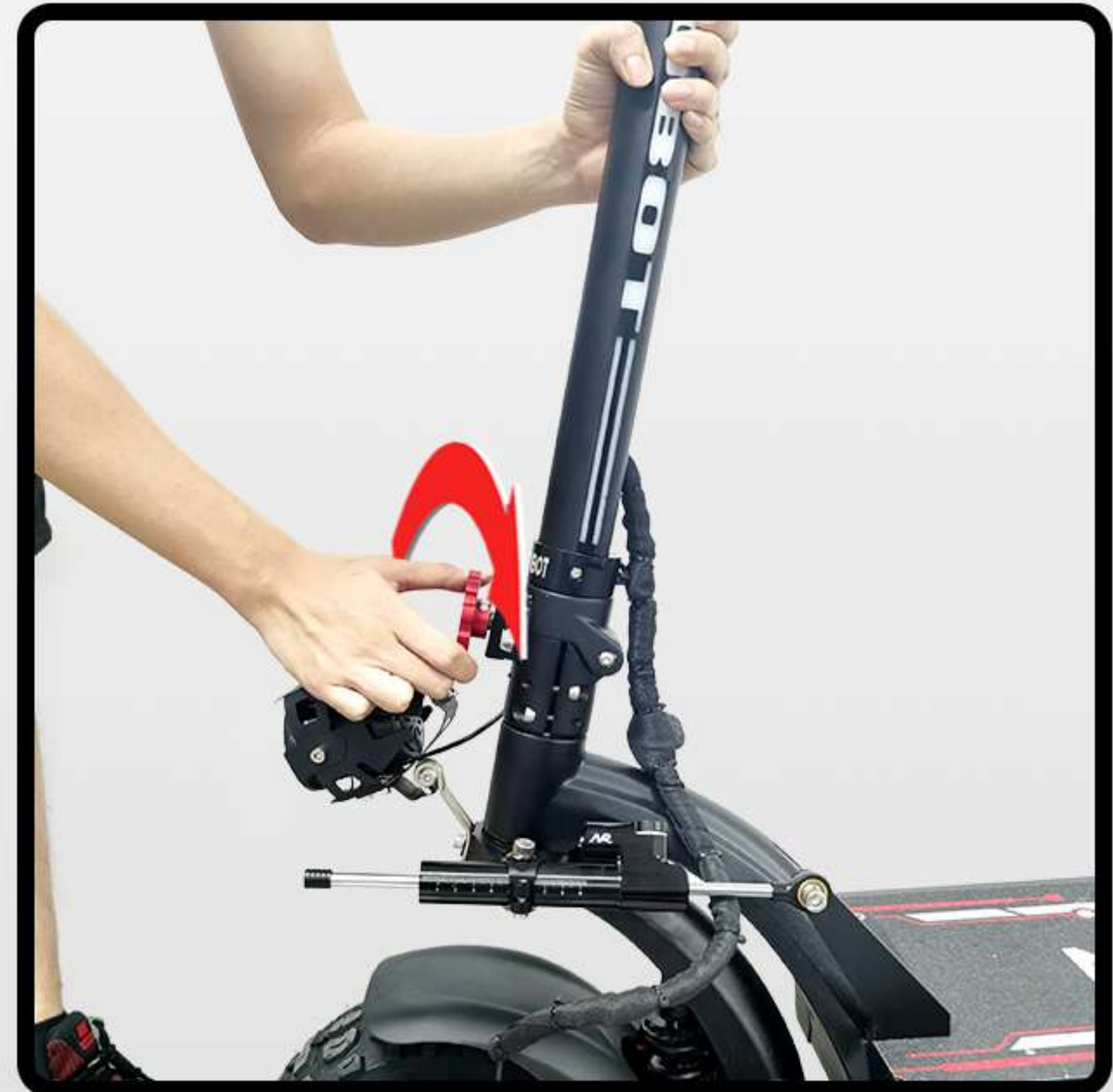
② Align the J -shaped buckle with the grooves, then tighten the folding knob.
