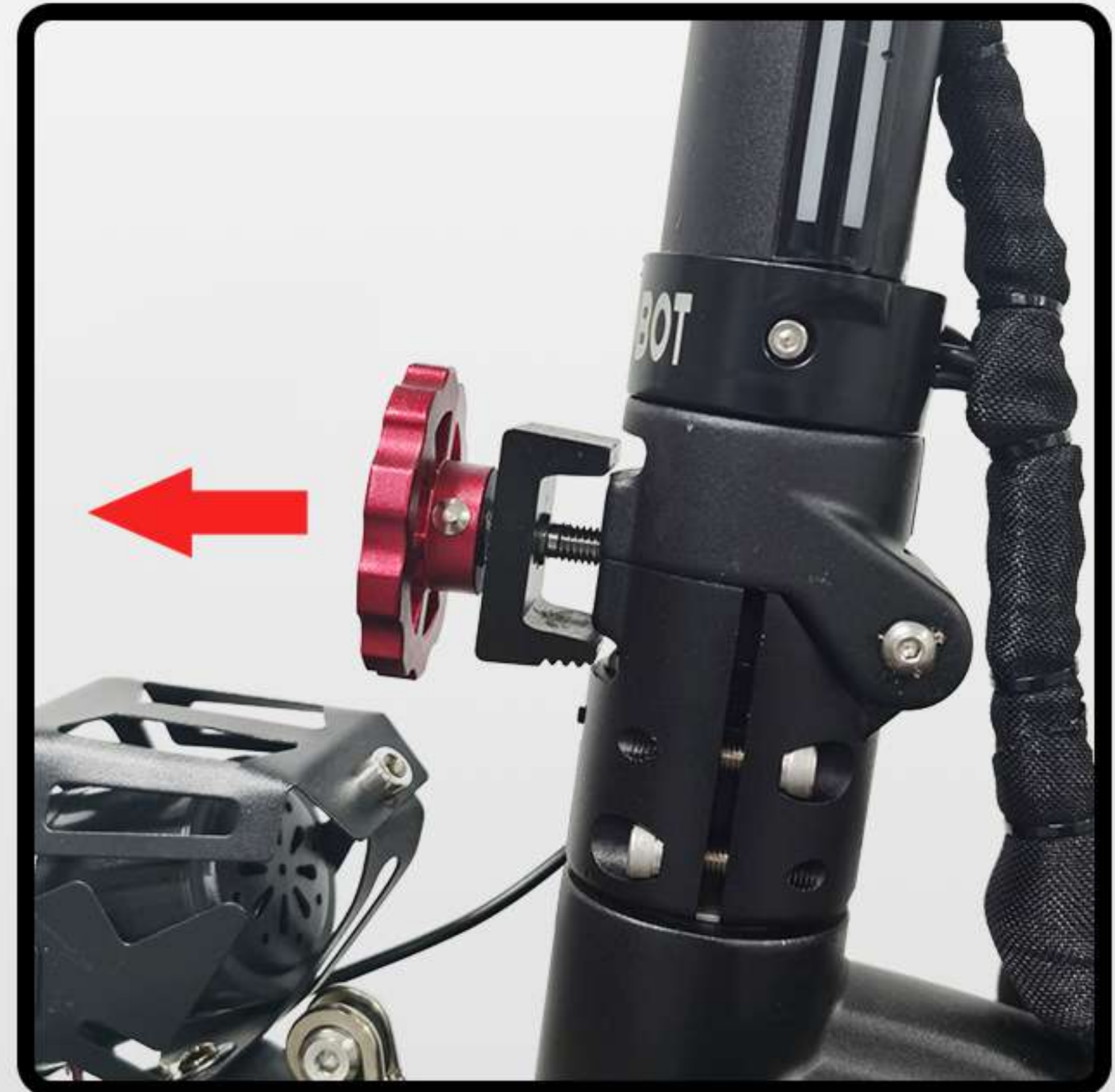
② Keep loosening the folding knob until the J-shaped buckle completely leaves the grooves
