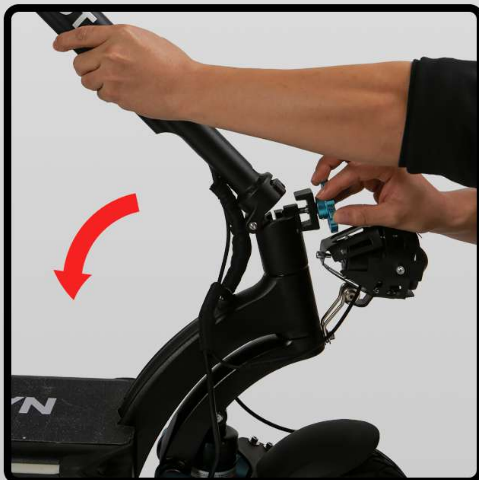
③ Lower the handlebar.
