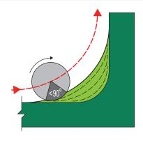
Generating an inside part radius with a smaller tool and a sweeping action creates a very desireable machining condition. The manageable radial depths of cut and smaller tool diameter allow management of the tool engagement angle, higher feed rates and better surface finishes. As the cutter reaches full radial depth its engagement angle will increase, but feed reduction should be much less than the other conditions listed above.
