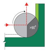
Generating an inside part radius that matches the radius of the tool at a 90° direction change can make for a less than ideal machining condition. With the tool experiencing extra material to cut (light green), increased engagement angle and a direction change some of the common results will be chatter, tool deflection/breakage & poor surface
