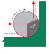
Generating an inside part radius that matches the radius of the tool with a sweeping direction change creates a machining condition a bit more acceptable. The smaller radial depths of cut in this example help to manage the angle of engagement, but at the final pass the tool will experience a very high engagement angle and again, a less than desireable machining condition. Some of the common results will be chatter, tool deflection/breakage and poor surface finish.
