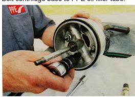
**Step 4**Lube the oil filler tube.
