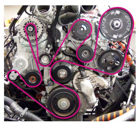
Step 8: Install the new Serpentine Belt as shown.
