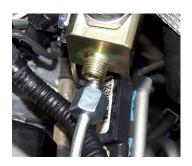
**Step 16:** Install the Hard fuel line from the CP3 to the Junction Block.
