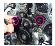
Step 6: Install new belt pulleys. (Box 1, item 10, 11, 15, 22) (Box 2, items 2, 6, 9, 16)
