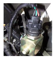
**Step 14:** Install the fuel sensor to the Fuel Junction Block.
