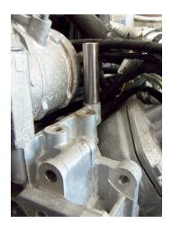
Step 4: Install CP3 Bracket Spacer to the A/C compressor mount. (Box 2, item 16)
