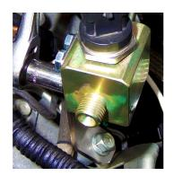
Step 13: Install the Fuel Line Junction
