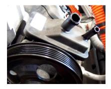
Step 1: Install the new PPE updated Power Steering Reservoir from the kit on your OEM steering pump using clips and O-Ring. (Box 3, item 10, 11, 12)
