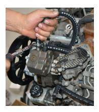
**Step 11:** Route the CP3 feed line under the throttle valve, on top of alternator.
