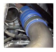
**Step 16:** Reinstall the driver side intercooler tube.
