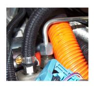
Step 15: Install the Hard Fuel Line from the back of the fuel rail to the Fuel Junction Block (only fingertight for now) (Box 3, item 9)
