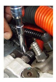
Step 10: Fit fuel line with hose clamps and install on to PPE 3/8" fitting on the CP3 fuel feed and return lines.
