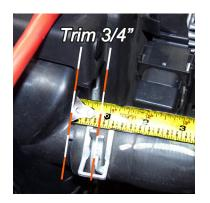
Step 27: Remove upper radiator hose and trim off 3/4" from the driver side where it mounts to the radiator to make clearance for the Dual Fueler pulley.
