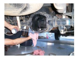
**Step 5:**Use a quality silicone (RTV) sealer. Apply an even bead on the flange around the holes as shown.
