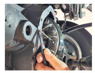
**Step 3**Apply a continuous bead of silicone (RTV) on flange surface and around bolt holes.
