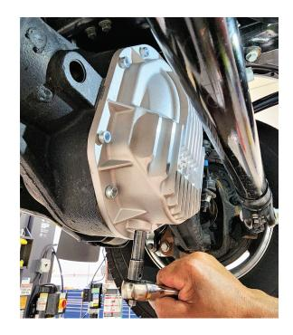
**Step 7**Replace and tighten Fill Plug to 18-22 lb-ft.
