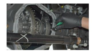
**Step 3**Apply a continuous bead of silicone (RTV on florge surface and
