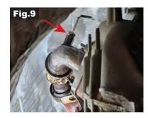
To remove the exhaust back pressure sensor tube, start by loosening the nut that holds the bracket in place. After that, loosen the flare nut that secures the tube. Next, detach the tube from the up-pipe and set it aside. Fig.10
