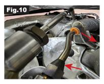
Step 10. To remove the up-pipe loosen the 11mm nut that secures the v-band clamp. Once loosened, carefully detach the clamp. Next, proceed to remove the three 13mm nuts securing the up-pipe to the manifold. Fig.11
