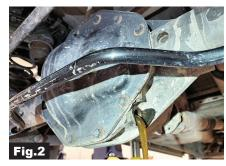
Thoroughly clean old sealant and fluid from the pan housing mating surface. Fig.3
