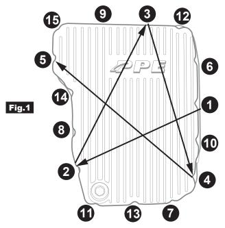
Step 6. Tighten NPT snug. Tighten drain plug to 18-22 ft lbs.
