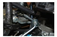
Remove stock FUEL FEED LINE from fuel filter housing and replace with the PPE fuel feed line provided in the kit.
