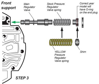
Install new YELLOW Pressure Regulator Valve spring.
