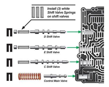
Install the three PPE white springs on to the D, E and C Shift Valves.
