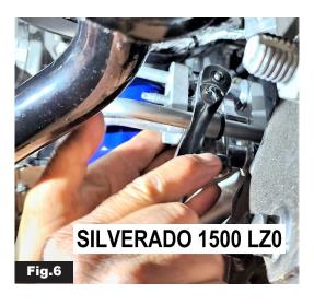
Step 7. Install the PPE Trans Thermal Bypass Valve using factory bolt. Fig.7-8
