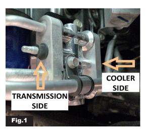
Step 3. Remove the retaining block and lines from the transmission side. Fig.2
