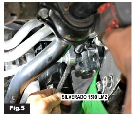
For LZ0 equipped vehicles, this bolt will also release the bracket securing the transmission fluid return line
