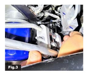
Notice LZ0 plate has block off as shown, ensure proper factory orientation is retained when securing to PPE bypass valve.
