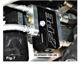
Step 9. Install the retaining block and lines from the transmission side with supplied M8 bolt.
