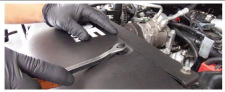
**STEP 1**Remove retaining clips and radiator cover.
