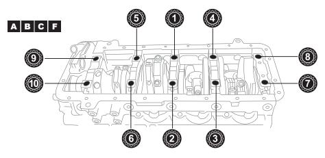
Lubricate Flat Washers (E) and M12 Cross Bolt (D) threads with Lubricant (F). Install Flat Washers (E) on to M12 Cross Bolts (D). Thread assembly into the block. Tighten M12 Cross Bolts to torque spec = 90 ft lbs.
