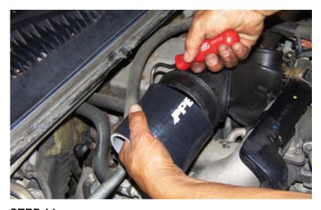
**STEP 14**Fit the silicone hose to the intake duct.
