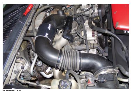
**STEP 15**Fit the other hose into the open end of the cut air box hose.
