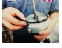
**Step 5**Install oil filler tube using stock bolt.
