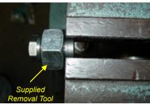
Step 6. Another view of removing the valve cap after loosening in step 5.
