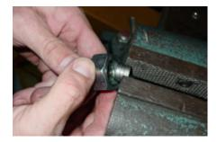
Step 7. Remove the metal spring, then insert the two supplied metal shims into the valve. 3 shims are supplied with the DURAMAXIMIZER, however only 2 need to be used.
