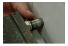
Step 8. Replace valve spring and then cap. Note that there are 3 holes in a triangle position on the inside of the valve cap that does not need to be removed from cap and should face towards the spring as it did when it was removed; hole alignment is not necessary.
