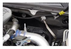
Step 3. Fuel Pressure Valve can now be seen after removing the glow plug controller assembly. Unscrew valve and remove from fuel rail.
