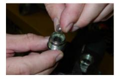
Step 9. Place the valve back in the vice, now place a thick piece of cardboard (or piece of wood) behind valve cap to prevent damage to the valve seal surface. Tighten the vice so that the valve cap re-enters the valve until fully seated. No need to overtighten, just tighten until snug.
