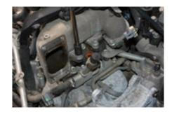
15. For LBZ models only: Remove top bolt from EGR cooler. For all other models remove all bolts.
