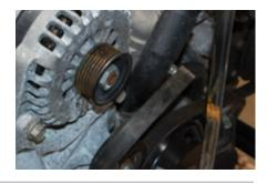
6. Disconnect power cable and plug from alternator.
