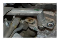
20. Disconnect high-pressure fuel line and remove stock rail fitting.
