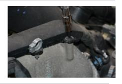
11. Remove Allen screws and nuts from air intake heater.
