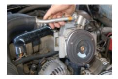
Remove opposite end of the highpressure fuel line with a 17mm flare nut wrench. Set aside. The factory fitting will now be visible.
