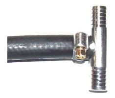
Route fuel line back to the pump. Secure with hose clamps.
