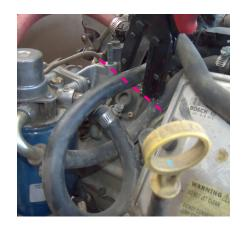
Install T fitting into fuel filter feed line. (Box 1, item 1, 7, 19)
