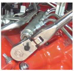
Use magnet to remove inner spacer plug as shown.
