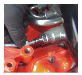
Reinstall AC Compressor using the stock bolts on the left side.
