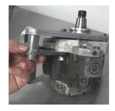
Bolt top of Bracket to AC Compressor. NOTE: One bolt from AC Compressor will be reused to secure lower bracket. Install washer between the bottom bolt and bracket to ensure the pump stays straight and secure. (Box 1, items 11, 21)
