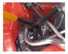
Install assembled T Fitting and hose and tighten hose clamps.
