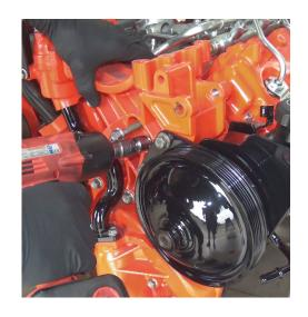
Use Torx FXT 500E wrench and a breaker bar to break tight seal and remove Fuel Rail Plug.
