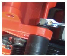
Spacer bushing should be flush
