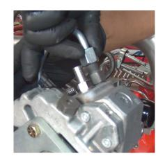
Install Return Line. Tighten clamps. (Box 1, items 3, 20)
