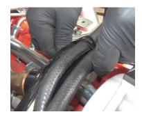
Install Duel Fueler Pulley using 18mm washer and nut (supplied). (Box 1, items 8, 9, Box 3, item 2)
