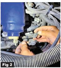
Step 3: Disconnect the WIF (water in fuel) sensor from the harness. (Fig 2.)
