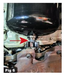
High-Capacity Premium Efficiency Fuel Filter
