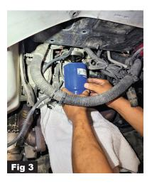
Step 4: Remove the old filter and clean the mating surface around the housing. Inspect the fuel filter housing flange to ensure that all old O-rings have been completely removed and have not adhered to the surface.(Fig 3.)
