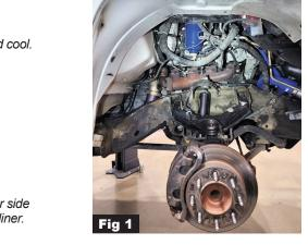
Step 2: Remove the passenger side wheel and wheel well liner. (Fig 1.)
