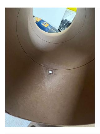
After the CA dried and is sanded I insert the screw through the hole in the couple and thread the t-nut on to the inside of the coupler. I then mix up some epoxy and epoxy the t-nut to the coupler. Let this set for about 30 minutes.
