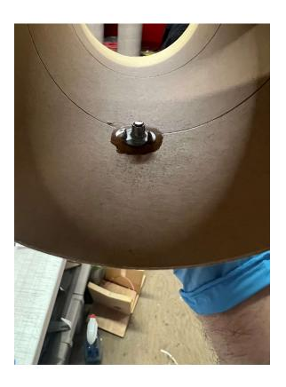
After the epoxy is hard I remove the screw and insert the coupler into the body tube. Align the hole up and insert the screw.
