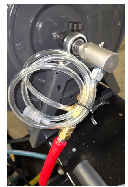
Chemical injector- connected to swivel of the hose reel. Injects the chemical while flowing at low pressure.
