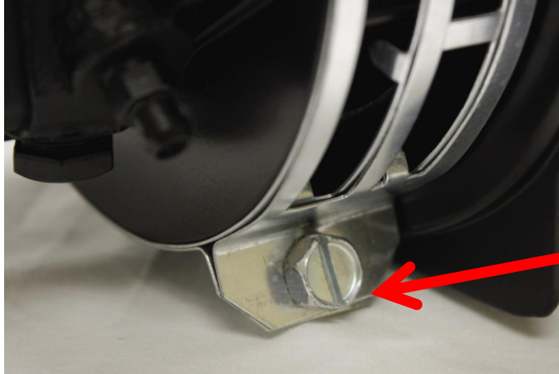
Figure 20– Air Band Adjustment Screw Location
